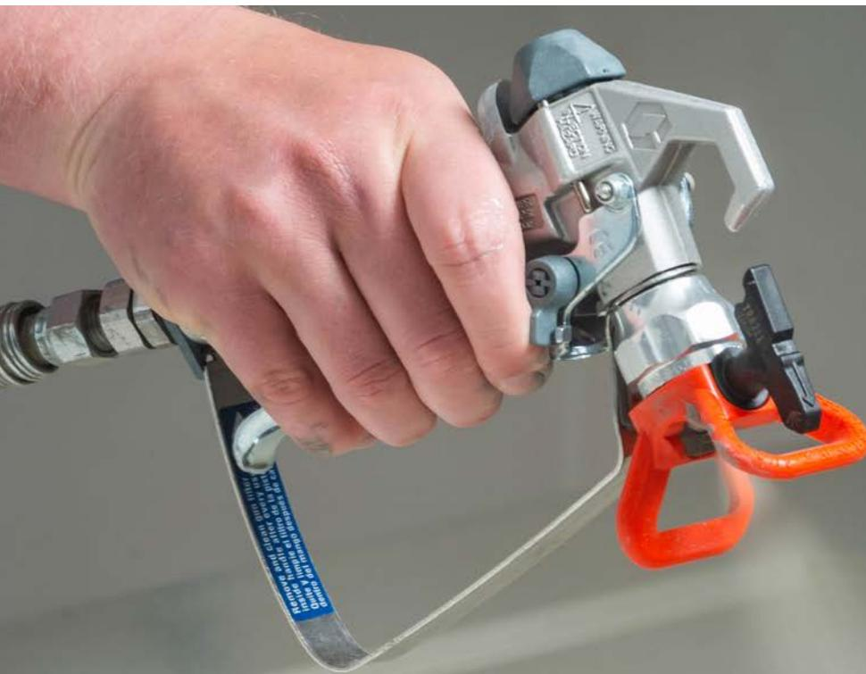
The spray tip tells the pump how hard it must work in order to maintain the required pressure. It ensures that the paint atomises under a certain fan width and flow rate – an effect similar to placing your thumb on the end of a garden hose.
